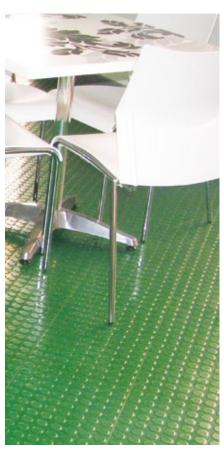
for easy cleaning, and provides excellent non-slip characteristics, which makes them particularly suitable for wet areas such as in change rooms. Transit tiles do not absorb mineral oil-based liquids because they are PVC-based, and they are also impervious to most solvents and chemicals.
